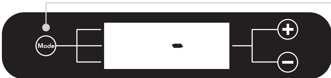
Once the product is switched on, the appliance will set the recommended temperature for the fridge compartment on the display +5°C. For the freezer compartment, the product will automatically set the freezer to the recommended temperature of -18°C.
