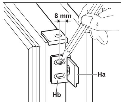
11. Remove the brackets and mark a distance of 8 mm from the outer edge of the door where the nail must be fitted (K).
