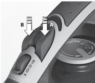
**4. Using the spray mist and steam jet function.** Ensure that water tank is at least 1/4 full. Use spray mist to pre-dampen fabrics by pressing spray button several times to release a fine mist (A). To use the steam jet function, ensure that tank is at least 1/2 full. Press steam jet button several times to prime pump (B).
