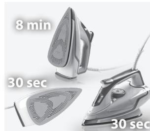
**6. 3-way Auto-OFF.** If iron is left unattended on soleplate or on the side, it turns off after 30 seconds. If left unattended on the heel, it turns off after 8 minutes. To turn on, just begin to iron again. The indicator light will flash yellow and the sound alert will beep 6 times before Auto-OFF.
