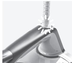
**3. Plug power cable into a power outlet.** Power indicator light turns on. Set temperature by turning temperature selector to adequate choice. When the light turns green, the iron is ready to use.
