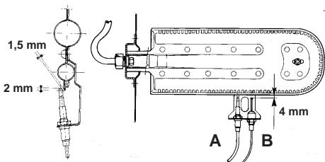
**A** =TERMOCOPIA / THERMOCOUPLE / THERMOCOUPLE
