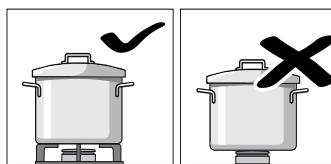
Do not place large pans on the burners near the control knobs. These may be damaged by the very high temperatures.
