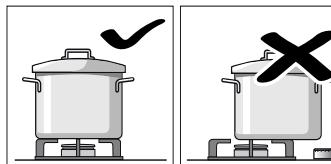
Always centre the pan over the burner, not to one side. Otherwise it could tip over.
