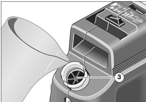
When filling, take care that the grid over the rubber surge protector 3 is not pressed in by the filling container.
