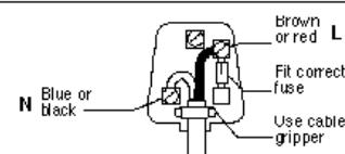
Neither core is to be connected to the earth terminal of a three-pin plug.
