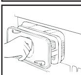
4. Gently remove any dust or fluff with a cloth, then wash the unit by holding it under a running tap turning it so that water flows between the plates, to remove any dust or fluff.
