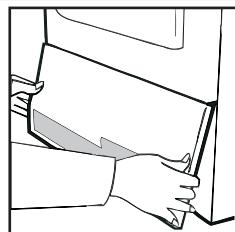
2. Pull firmly on the handgrip and slide the water container out of the dryer.
