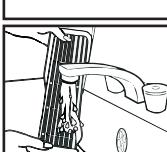
5. Check the gasket position after cleaning. Fit the gasket in to the groove if it is misaligned.
