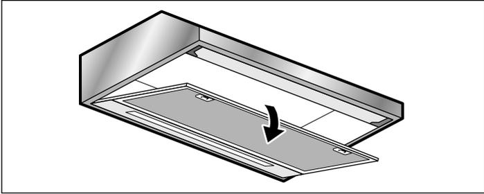
3. Position the filter grid at an angle and remove it.
