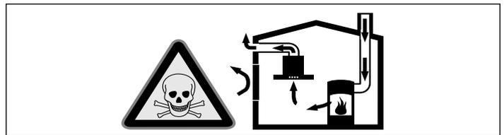
Room air-dependent heat-producing appliances (e.g. gas, oil, wood or coal-operated heaters, continuous flow heaters or water heaters) obtain combustion air from the room in which they are installed and discharge the exhaust gases into the open air through an exhaust gas system (e.g. a chimney).
