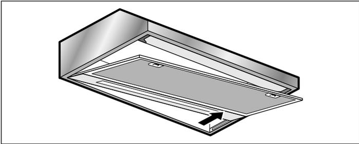
4. Remove the wires and then remove the fleece grease filter.
