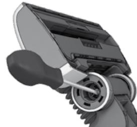
3. Unscrew the wheel axis and clean all parts.
