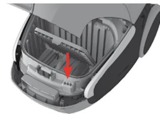
8. Replace or wash the motor filter when dirty or after every 5th s-bag. Push the filter holder down and pull it out. Exchange the filter or wash it, see step 9.
