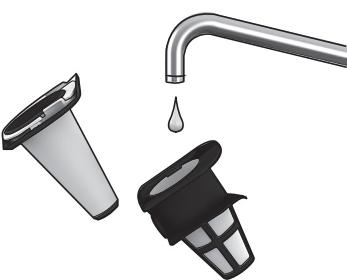
**4b.Separate both filters.** Dust container and filters can be shaken clean or rinsed in warm water (never in dishwasher). All parts must be dry before reassembled in reverse order.
