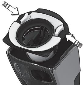
**4a.Cleaning of dust container and filters.** (Recommended every 5th cleaning). Release dust container, take out both filters by pressing release buttons.
