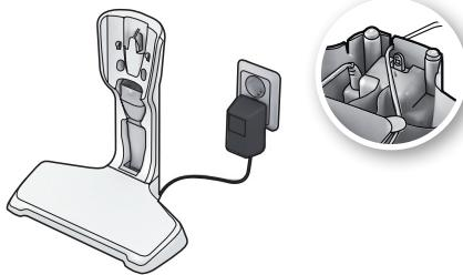
1. Position the charging station well away from heat sources, direct sunlight or wet places. Insert the adaptor into the mains and connect it to the charging station.
