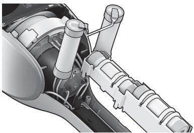
2. **Cut the connecting cables,** remove the batteries, put tape over the visible metal areas. Place batteries in suitable packaging.
