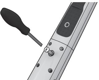
2. Secure the handle by tightening the locking screw supplied. Use a screwdriver or a coin.
