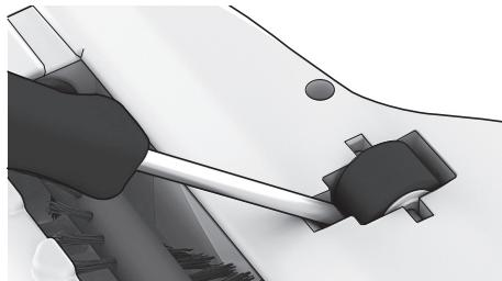
2. **If the wheels needs to be cleaned,** remove them carefully by using a small screwdriver.
