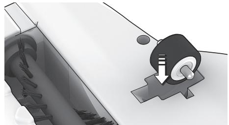
3. **Remove objects that may have become jammed** in the wheel shafts. Reassemble the wheels by pressing them back into their tracks.
