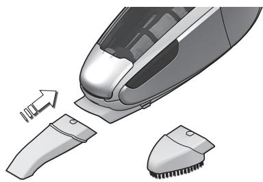
2. Attach the crevice nozzle to facilitate cleaning of areas difficult to reach, or attach the brush for dusting.
