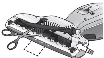
2. **Lift out the brush roll and clean it.** Use a sharp object to remove threads. Reassemble the roll, making sure it can spin freely. Close hatch cover.
