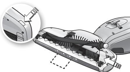
1. **First turn Ergorapido off.** Push the brush roll release button. The hatch cover will come slightly free and the brush roll can be removed.
