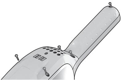
1. Batteries should always be run flat before removed. **Ergorapido must be disconnected from the charging station when removing the batteries.** Undo the screws. Carefully lift the hood.
