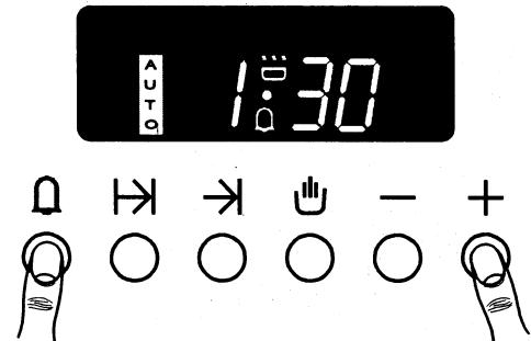
Press the "Short time **9**" key. A suggested time of 0:00 appears in the timer display. Press the **PLUS 13** key to program the required time. In addition to the "Pot **6**" symbol, the "Bell **7**" symbol also lights up in the display. The elapsing short time is displayed in the timer.
