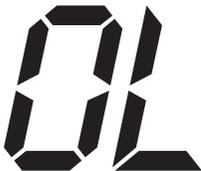
If the code appears, step off the scales to avoid damage.
