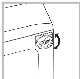
2. If the floor is uneven, the front feet of the machine may be adjusted until it reaches a horizontal position (the angle of inclination must not exceed 2 degrees).
