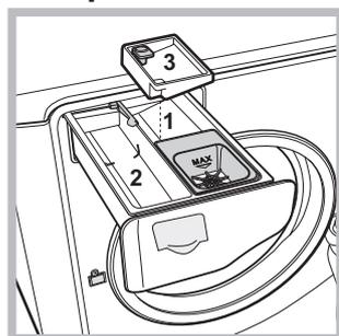
This option offers a high-performance wash due to the greater quantity of water used in the initial phase of the cycle, and due to the increased wash cycle duration, is particularly useful for the removal of stubborn stains. It can be used **with** or **without** bleach. If you desire bleaching, insert the extra tray compartment (3) into
