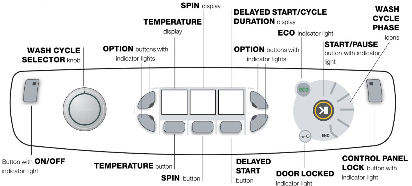
Button with **ON/OFF** indicator light: press this briefly to switch the machine on or off. The green indicator light indicates that the machine is switched on. To switch off the washing machine during the wash cycle, press and hold the button for approximately 3 seconds; if the button is pressed briefly or accidentally the machine will not switch off. If the machine is switched off during a wash cycle, this wash cycle will be cancelled.
