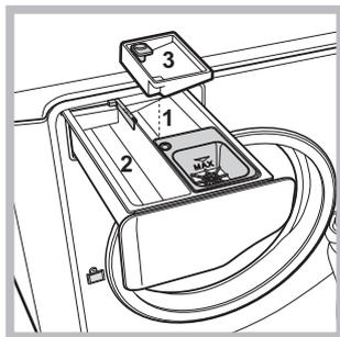
**To bleach laundry without carrying out a full wash cycle**, pour the bleach into the extra compartment 3, select the "Rinse" cycle and activate the "Super Wash" option .
