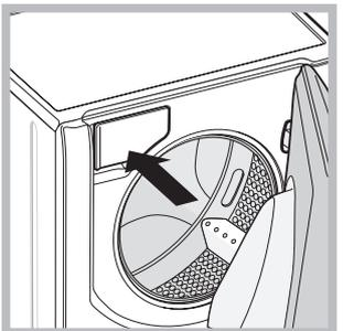
The detergent dispenser drawer is located inside the machine and can be accessed by opening the door.
