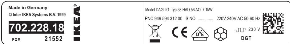
The graphic above represents the rating plate of the appliance (without serial number which is generated dynamically during the production process), which is located at its underneath surface of the casing.
