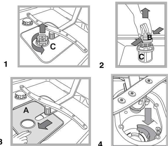
After cleaning the filters, replace the filter assembly and fix it in position correctly; this is essential for maintaining the efficient operation of the dishwasher.
