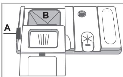
Introduce the detergent into the dry dispenser "B" only. Place the amount of detergent for pre-washing directly inside the tub.
