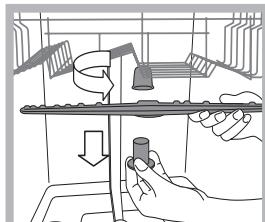
To remove the upper spray arm, turn the plastic locking ring in an anti-clockwise direction. The upper sprayer arm should be replaced so that the side with the greater number of holes is facing upwards.
