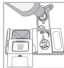
1. Open the dispenser "D" by pressing and pulling up the tab on the lid;
