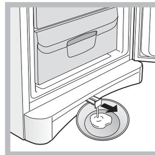
4. Certain appliances are fitted with the DRAIN SYSTEM to lead the water outside: insert the scraper into the slot provided at the bottom and let the water flow into a container (see diagram).
