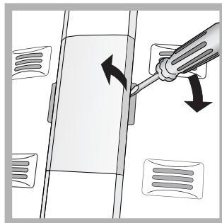
To replace the light bulb in the refrigerator compartment, pull out the plug from the electrical socket. Follow the instructions below. Access the light bulb by removing the cover as indicated in the diagram. Replace it with a similar light bulb within the power range indicated on the cover (10W).
