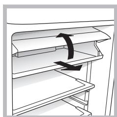
**COOL BOX:** for fresh meat and fish. Due to the compartment's low temperature (the coldest in the refrigerator) and to the clear door that provides protection against oxidation and blackening, food can be stored for even up to one week. It can also be used for "cold meals."
