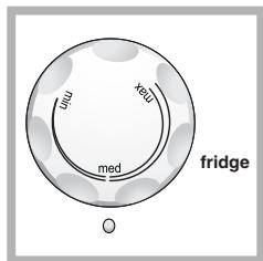
The temperature inside the refrigerator compartment automatically adjusts itself according to the position of the thermostat knob.
