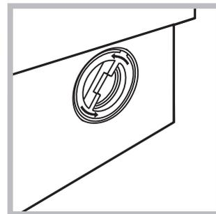
2. unscrew the lid rotating it anti-clockwise (see figure): a little water may trickle out. This is perfectly normal;
