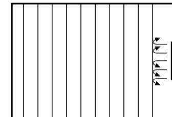
The washing facing the drier obstructs the flow of air so that the washing towards the back takes much longer to dry.
