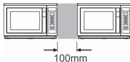
Note: 100mm clearance is required between two ovens side by side
