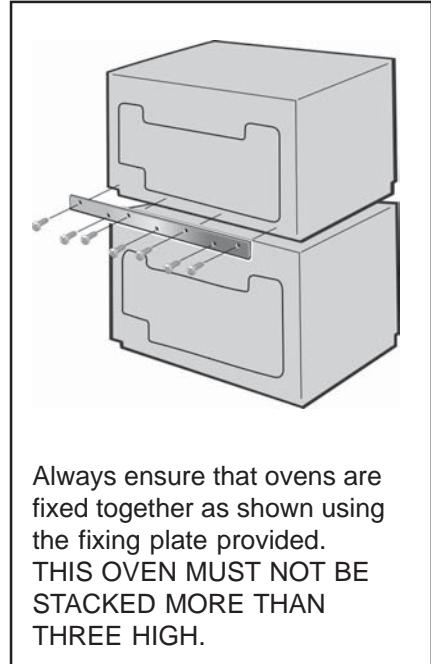
Always ensure that ovens are fixed together as shown using the fixing plate provided.
