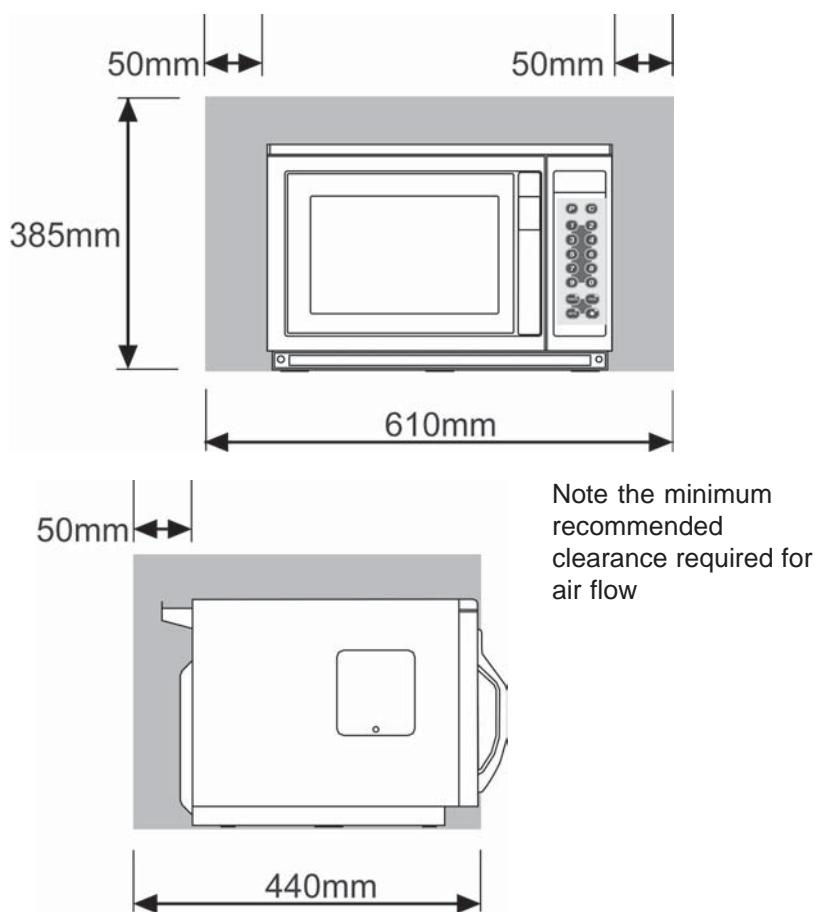
Note the minimum recommended clearance required for air flow
