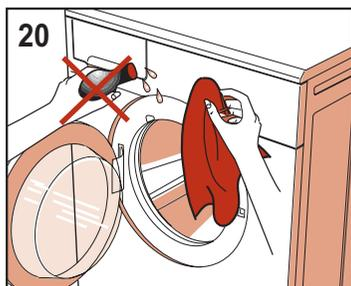
**WARNING!!** Never use chemicals, abrasive products, alcohol, soap, petrol or other solvents to clean the appliance as these may cause damage. (fig.20)
