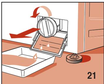
Place a cloth or flat plate under the filter to collect any water that may still be inside it. Open the filter door, unscrew the filter and remove it, turning in an anticlockwise direction (fig.21).
