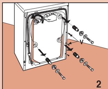
Block off the holes with the plugs provided, which can be found in the bag containing the documents.
