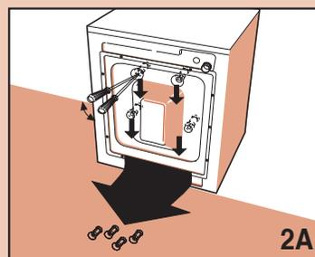
Insert a screwdriver in the holes and proceed as shown in the figure to recover the 4 plastic spacers.
