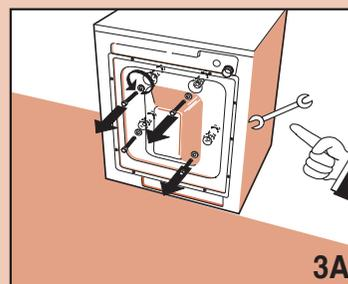
**N.B. If the spacers fall into the inside of the machine, open the rear panel, recover them and then replace the panel.**
