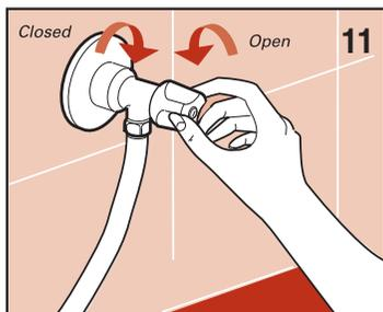
connection to the water supply) and the supply tap is open.
