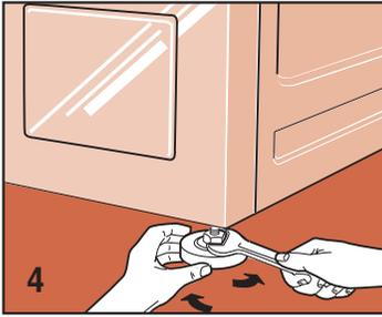
After selecting a suitable position, level the machine carefully using the adjustable feet (Fig. 4). Particular care must be taken when selecting the position, levelling the washing machine and ensuring the safety of lock nuts.
