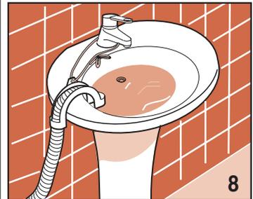
special bracket supplied and hook it over the edge of the sink or washbasin. Then tie the hose and bracket to a tap or similar (fig. 8). To avoid overflowing, the sink drain must be clear of obstructions and must be able to empty quickly.
