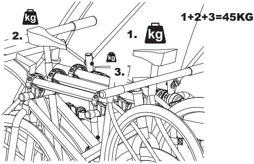
**B/ INSTALLATION DES SANGLES DE SECURITE / INSTALLATIE VAN VEILIGHEIDSSPANRIEMEN /
