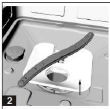
1. Turn the micro filter anticlockwise and remove it.
