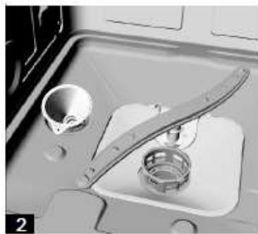
1. Remove the lower dish-rack and the lid of the water softener container.
