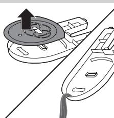
**10** Remove the drip tray cover and empty the drip tray.
