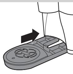
**13** Put the drip tray cover on the drip tray and slide the drip tray back into the coffeemaker.
