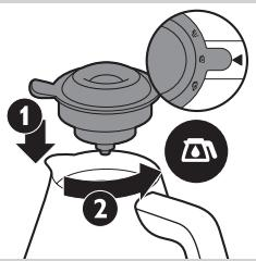
**5** Turn the lid of the jug by its lever to 'closed/brewing' position. In this position, the arrowhead on the jug handle points to the 'closed/brewing' symbol on the jug lid.
