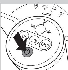
**4** Press the on/off button to switch on the coffeemaker.
