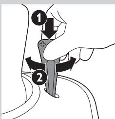
**8** For a coarser setting, push down and turn the grinding degree adjustment tool clockwise. For a finer setting, push down and turn the grinding degree adjustment tool anticlockwise.
