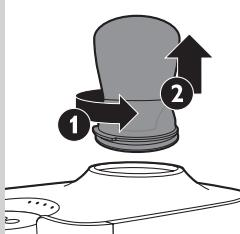
**2** Turn the bean-funnel anticlockwise to remove it.
