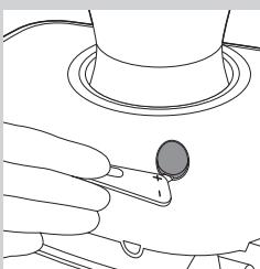
**6** Insert the lug on the broad end of the grinding degree next to the cap of the grinding degree adjustment hole and press lightly. This makes the cap open automatically.
