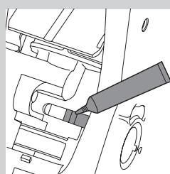
**6** Apply some lubricant on both sides of the lever in the brewing unit.
