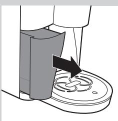
Empty and clean the water tank, the coffee grounds container and the drip tray every day. Also empty and clean the water tank and coffee grounds container when the 'water tank empty' light and/or the 'coffee grounds container full' light go on. Empty and rinse the drip tray when the 'drip tray full' indicator indicates the drip tray is full.
