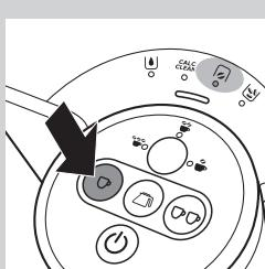
**5** Press the 1-cup button to start the rinsing cycle.
