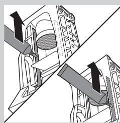
**4** Apply some lubricant around the shaft in the bottom of the brewing unit.
