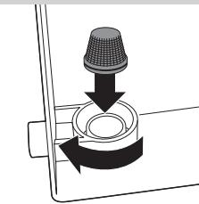
**4** Place the filter back in its holder by turning it a little while pushing it down gently.
