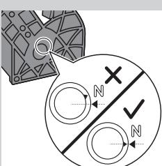
**8** Before you slide the brewing unit back into the coffeemaker, make sure the two reference signs on the side match. If they do not match, perform the following step:
