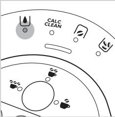
Note: The 'water tank empty' light goes on when there is not enough water in the water tank to brew one cup of coffee.
