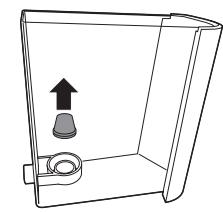
**2** Remove the filter from its holder in the water tank and rinse it under the tap.
