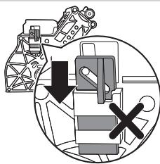
**9** Make sure that the locking hook of the brewing unit is in the correct position. The hook is not correctly positioned if it is still in bottommost position.
