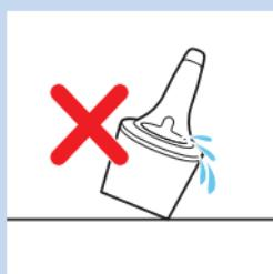
Do not tilt the SmartClean to prevent leakage.
