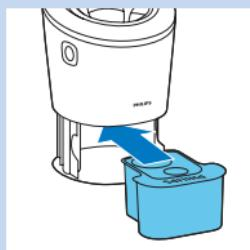
**5** Place the cleaning cartridge in the SmartClean system.
