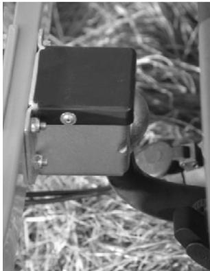
The bike carrier can be mounted with the coupler on the hitch ball of your car. Slightly tighten the big bolt (M16x90). Check if the carrier runs parallel to your car (or bumper of your car). Next, tightly screw the bolt down with the supplied key until the carrier can no longer move on the hitch ball.
