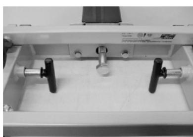
If you tilt the inner frame (you need to pull out and rotate the two locking pins, see explanation on page 36), it will be easier to put the mounting plate in its place and tighten the nuts! Turn the two locking pins back into the secure position to be sure the inner frame will not tilt while you are mounting.
