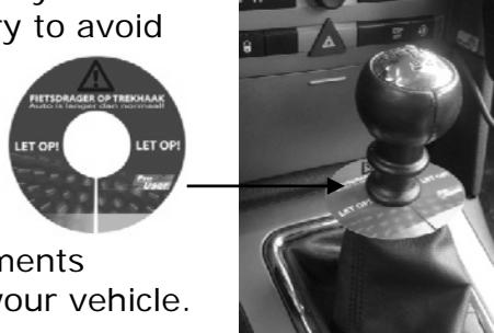
When you have a vehicle with electronic parking sensors, an error message can come when the bike carrier is mounted. Switch off the parking system during the use of the bike carrier.
