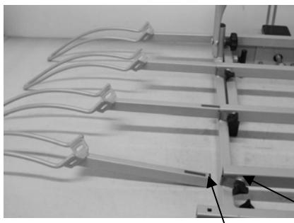
Slide the eight wheel holders into the openings in the base frame. Make sure to slide the wheel holders into the frame with the ends pointing downwards (see picture). Fasten the wheel holders using the plastic star knobs. When adjusting the wheel holders, they may not be pulled out beyond the red marking!
