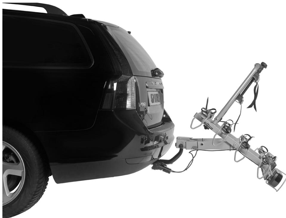
To secure the carrier again, you have to lift it and push the two locking pins back in. Subsequently you rotate the pins again by a quarter turn so the handles are vertical with the long part downwards. You will hear a click once they are secured.
