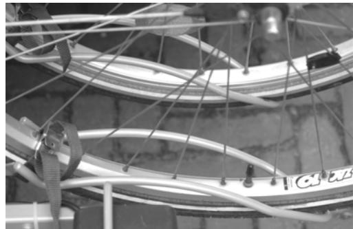
Secure the bike frame to the U-frame using the frame holder. Since the frame holders do not have to be used in a fixed point, you can try out several positions. It is important to place the frame holders as high as possible. Use the straps to secure the bikes. With these straps, any bike can be secured easily without placing a load on the bike crank!
