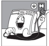
The power supply socket to which the machine is connected must be earthed and must comply with the safety requirements
