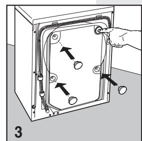
For transport purposes the swinging unit in the machine is blocked using 4 spacers with screws. Before starting the machine these screws must be removed using a screwdriver.
