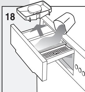
**Attention!** Never remove the detergent drawer when the machine is running, as water may come out of it.
