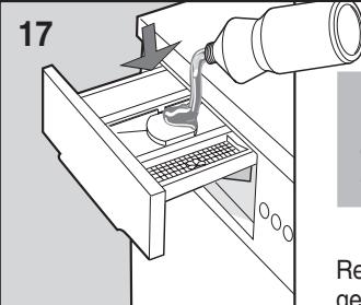
**N.B.** When using liquid detergent (recommended for programs that do not use the pre-wash cycle), insert the special container (if there is one) in centre compartment "2" (as shown opposite), then pour in liquid detergent up to the maximum level indicated.
