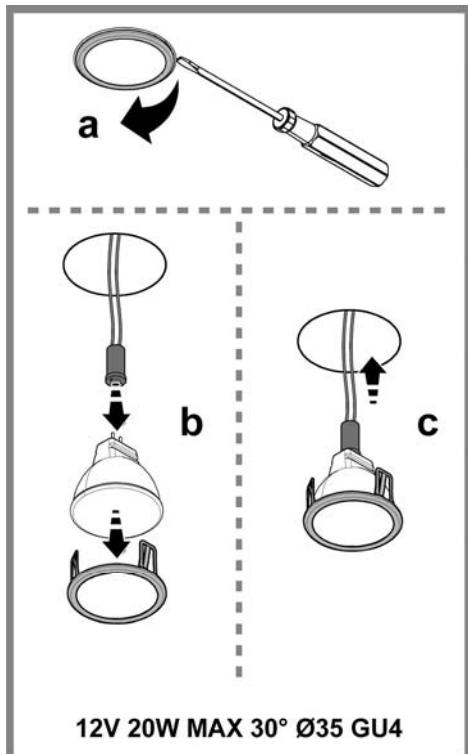
**Replacing lateral lamps.**
