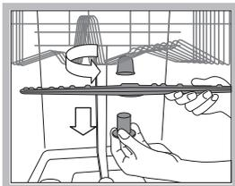
To remove the upper sprayer arm, rotate the locking ring in an anti-clockwise direction. The upper sprayer arm should be replaced with the holes facing upwards.
