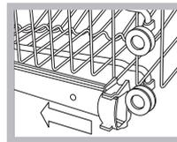
Open the left and right guide rail stops and pull out the rack; position it higher or lower as required, slide it along the guide rails until the front wheels are in place and close the stops (see figure).
