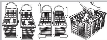
The modular basket may be separated into two parts, a solution which is recommended when performing a half
