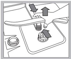
The lower sprayer arm can be removed by pressing on the side tabs and pulling it upwards.
