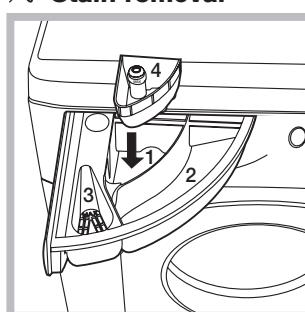
This function is particularly useful for the removal of stubborn stains. Place extra compartment 4 (supplied) into compartment 1. When pouring in the bleach, be careful not to exceed the "max" level marked on the central pivot (see figure). To run the bleach cycle on its own, pour the bleach into extra compartment 4, set the "Rinse" programme and activate the "Stain removal" programme. To bleach during a wash cycle, pour in the
