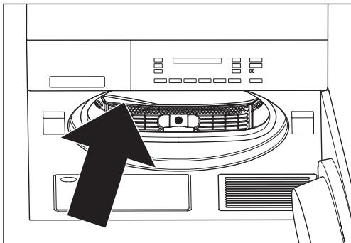
After longer operation, small deposits (lime, fabric refiner) can form on the front inner side of the drum on both sides of the longish moisture sensors. With moisture controlled programmes, this can result in the desired level of dryness not being reached.
