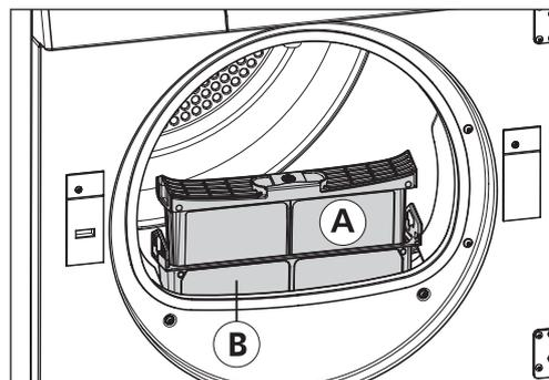
► Run the pipe of the vacuum cleaner or the brush around the well of the filter support.
