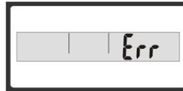
Over load indication. The weight subject on the platform exceeds the maximum capacity of scale Please step off to avoid damage.
