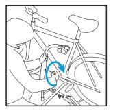
Place the bicycle with the handlebars to the left behind the stand and set the height by turning the knob completely out and turning it in again at the correct height.
