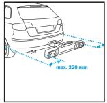
Width adjustment: press the red unlocking device and slide the light units out in steps of 1 cm.
