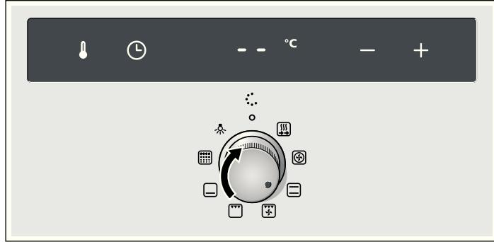
2. Set the temperature or required grill power using the + or - sensors.
