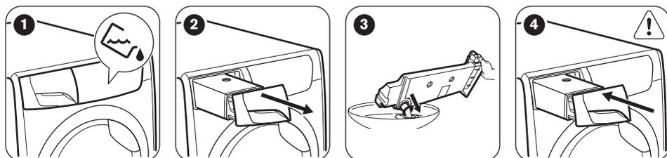
**i** You can use the water from the water container as an alternative to distilled water (e.g. for steam ironing). Before you use the water, remove dirt residues with a filter.
