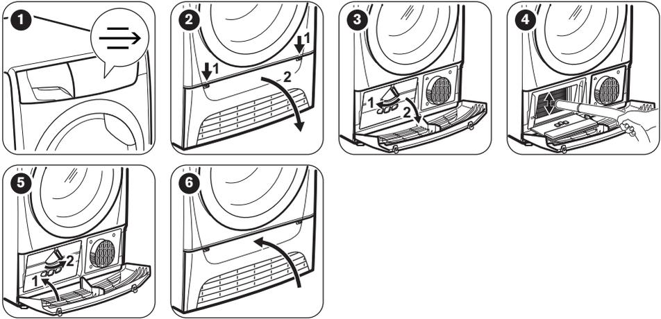
**4** if necessary, one time for each 6 months, remove the fluff from the heat exchanger compartment. You can use a vacuum cleaner.
